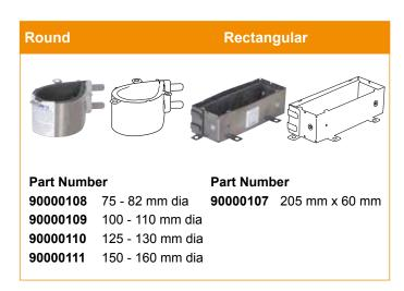
**Fire Collar** - prevents spread of fire, smoke and hot gasses where fire compartment wall / floor is penetrated by plastic pipes.
